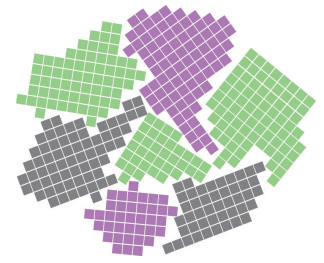
Grain boundaries. As a polycrystalline material solidifies, grains with irregular shapes form. The interfaces between grains constitute grain boundaries. (Squares represent unit cells within grains.)
