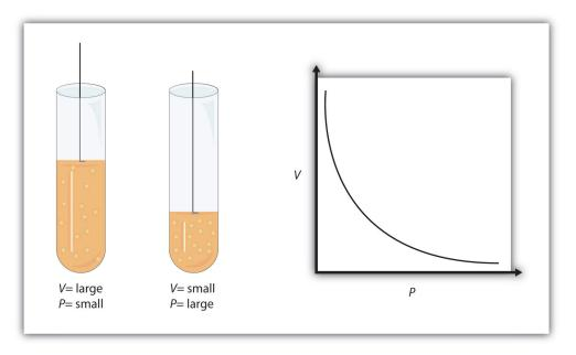
A piston having a certain pressure and volume (left piston) will have half the volume when its pressure is twice as much (right piston). One can also plot P versus V for a given amount of gas at a certain temperature; such a plot will look like the graph on the right.
