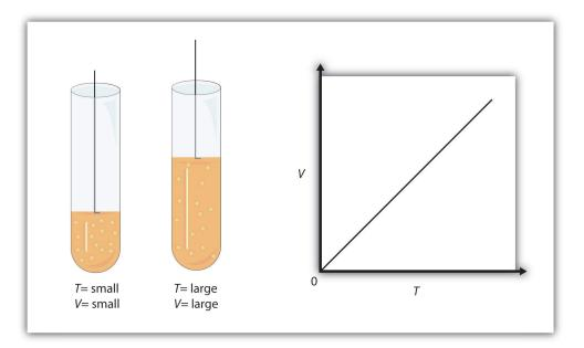
A piston having a certain volume and temperature (left piston) will have twice the volume when its temperature is twice as much (right piston). One can also plot V versus T for a given amount of gas at a certain pressure; such a plot will look like the graph on the right.
