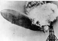
The German airship Hindenburg (left) was one of the largest airships ever built. However, it was filled with hydrogen gas and exploded in Lakehurst, New Jersey, at the end of a transatlantic voyage in May 1937 (right).
